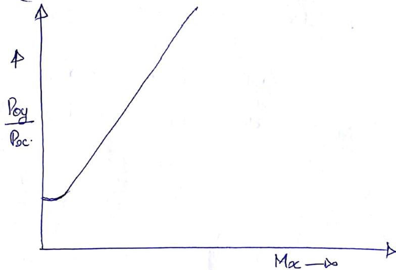
By obtaining the above plot we can easily obtain  $M_{0c}$  value for any given value of  $\frac{P_{0y}}{P_x}$ .
