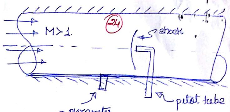
Placing a pressure tap upstream of pitot tubes position (such that it comes before shock) we can measure static pressure before shock. Hence from this step-up we can obtain  $P_x$  &  $P_{0y}$
